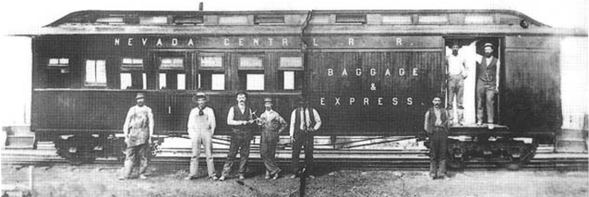
A fantastic view of the M&SV Combine #1, on the Nevada Central, rebuild with matchboard siding and Carters 4' trucks, circa 1897. Note the addition of the iron Queen Posts under the Needle Beams.
