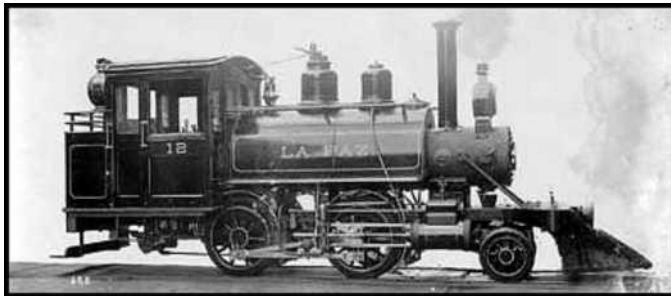
This 42" gauge loco for Nicaragua has unusual wheel arrangement for a saddle-tank engine.
