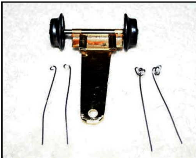
I substituted stainless steel spring material for the music wire. I also formed two separate springs, each mounted to the U bracket using 2-56 screws into tapped holes in the U bracket. Springs were formed with and without loops. The final springs used will be determined after testing. Two rectangular tubes to receive the spring ends are soldered to the top of the truck.
