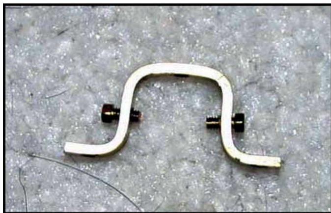
This U bracket for mounting the rear truck was formed using the techniques discussed by Vance in this section.
