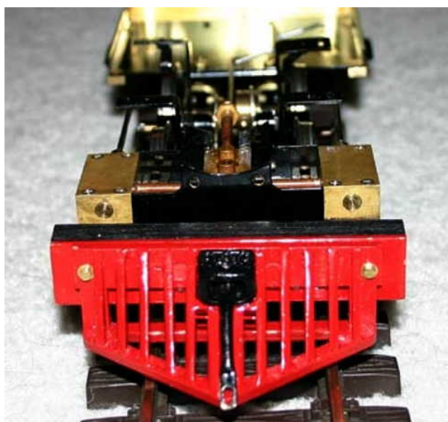
This shot shows the pilot mounted to the front beam which in turn is mounted to the engine frame.
