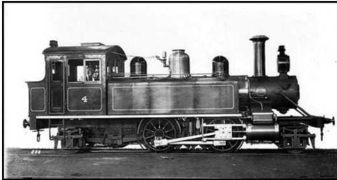
This 42" gauge loco, built for the Bantan Rly. in Japan, was a 2-4-2 Baldwin with side tanks and a rear bunker.
