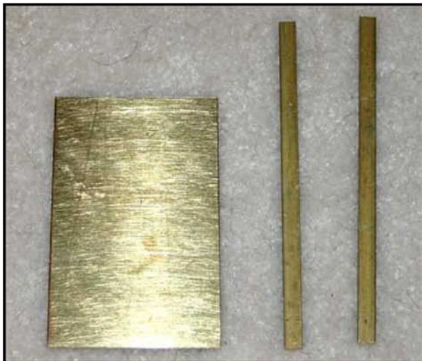
The two pieces of 1/8 x 1/4 inch bar stock are shown on the right. The sheet brass is shown on the left.
