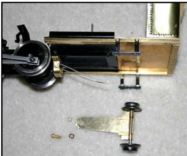
In this photo springs are mounted to the U bracket. A 0.1" piece of brass 3/16" tube acts as the bearing between the U bracket and the truck and prevents the truck from being pinched when the screw is tightened. The hole drilled in the truck is slightly oversized, allowing the truck to tilt vertically to deal with grades. The screw is a 6-32 brass screw with lock washer.
