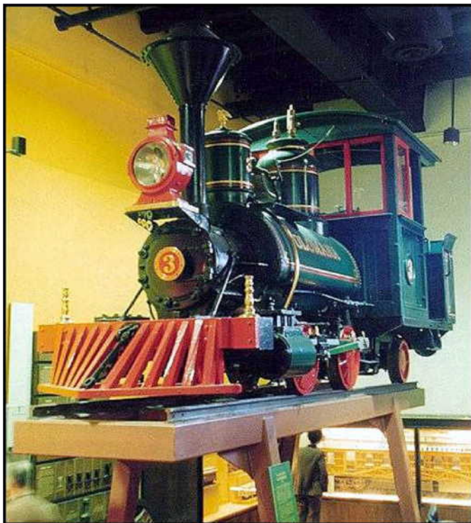
Note, however, that the windows are the same height on the front and sides of the cab. This cab has an open rear, a feature that will make it easy to get to the controls of a live steam engine.
