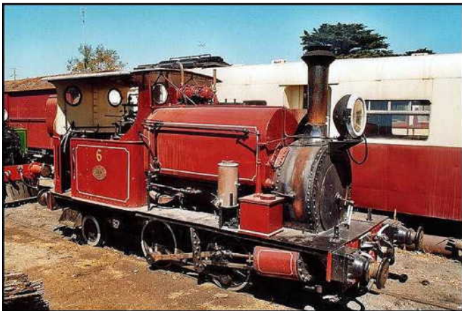
The example shown here is a typical 1903 Hudswell Clarke 0-4-2T, very similar to the designs used in Tasmania. This 42" gauge loco was used in the Portland Cement factories of southern Victoria. She is now in operating condition at the Ballarine Peninsula Railway, close to my home, and had always been a childhood favorite. A very similar 2ft gauge version of this loco, also resides at the Puffing Billy Narrow Gauge Museum, originally used on the Queensland Sugar cane tramways.
