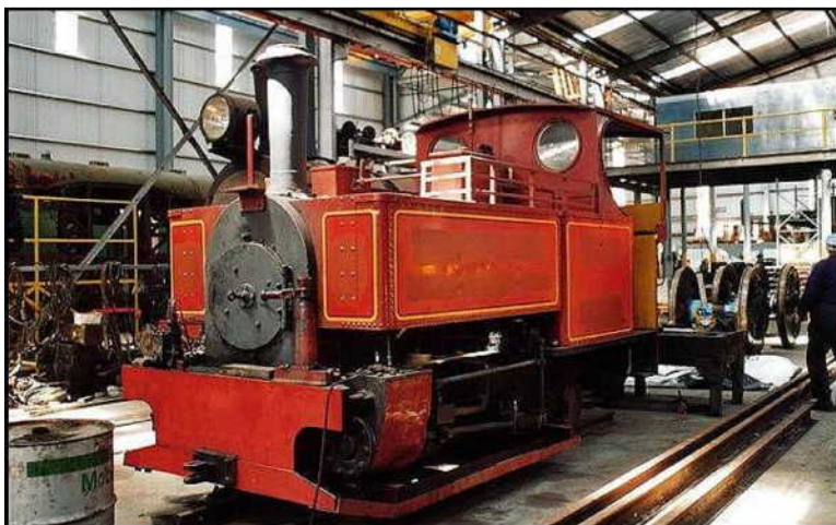
The Hunslet being readied for service for her new life at Sheffield, Tasmania. Note the environmental oil collection trays fixed under the side rods and cylinders.
