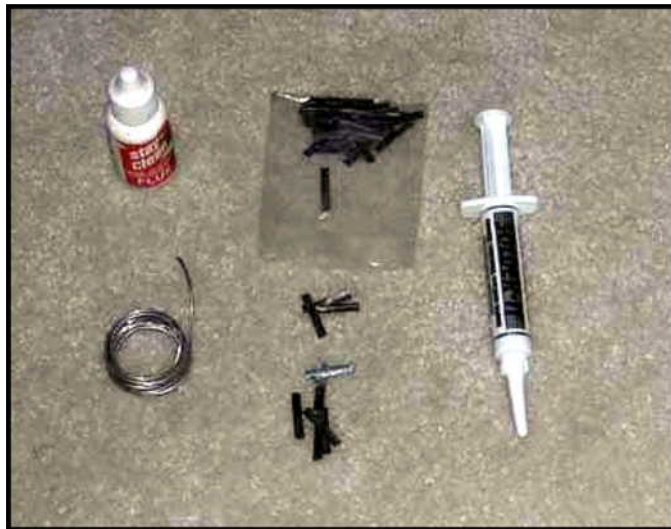
Left to right is silver solder with flux from Micro-Mark, ribbon solder from Radio Shack and paste solder in a tube, also from Micro-Mark.
