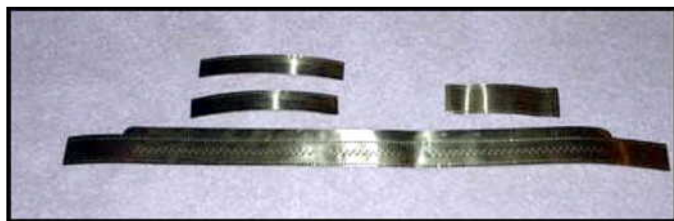
Top left is the two oil tank side panels. Top right is the oil tank top. On the bottom is the tender side outer shell.
