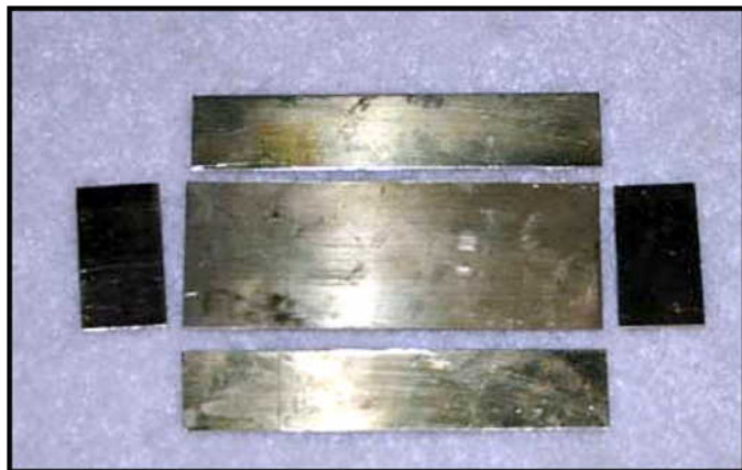
End walls (opposite ends), side walls (top, bottom) and tank top have been cut out and sized in this photo.
