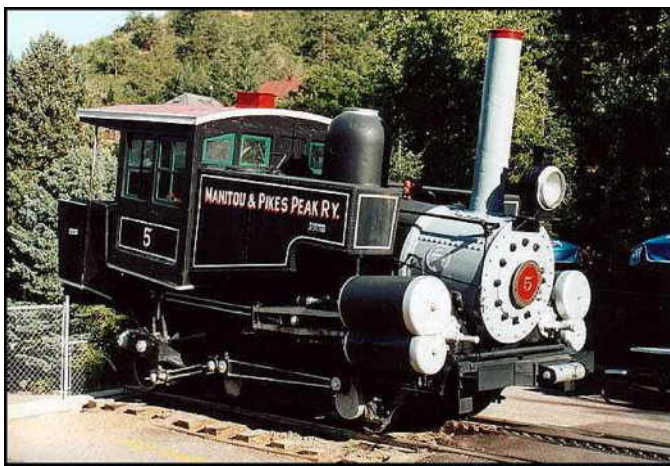
The typically Crooked Abt Mountain locos, this is one of the beautiful steam locos built by Baldwin, for the Pike's
