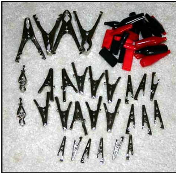
Looking for cheap metal clamps to hold your work together while soldering? This set of electrical clamps cost $5 at Harbor Freight. There were 28 in the package.
