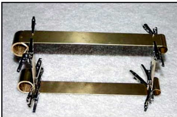
This shows the inner walls clamped together just prior to being soldered. Pipes being used to form the rounded corners are a 1" OD brass pipe and a .56" OD K&S tube. See the parts list for more information.
