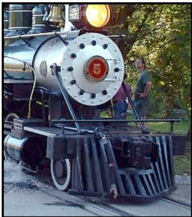
This front shot shows the pilot and coupler. The pilot is similar to the pilot shown in No. 5's original Baldwin builders photo.
