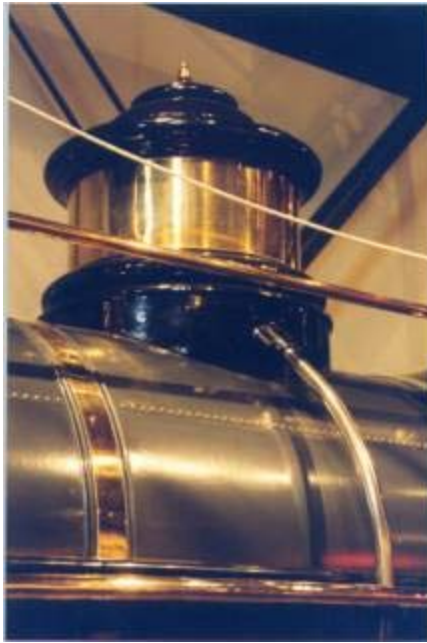
The sand dome of V&T #12, Genoa, 1873, Baldwin 4-4-0, made from cast iron with brass cladding. Cal State RR Museum, Sacramento
