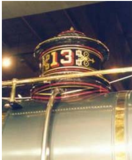
The sand dome of V&T #13 'Empire', 1873, Baldwin 2-6-0, made from cast iron and iron tubing. Cal State RR Museum, Sacramento.
