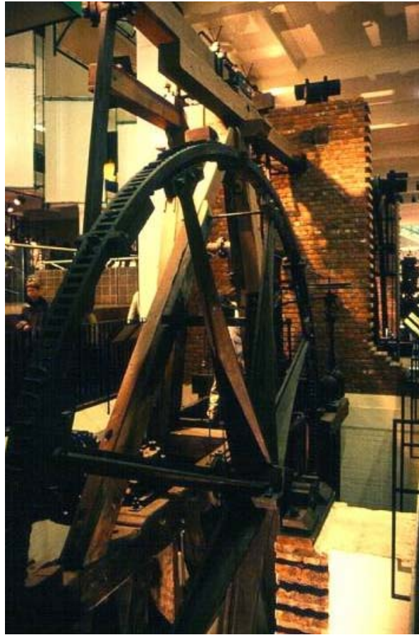
An early Boulton & Watt Steam engine. The big wheel is the first form of steam powered circular motion and also acted as a 'fly wheel' London Science Museum, UK.
