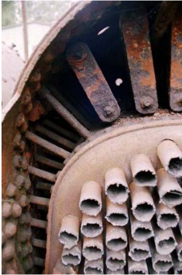
In this view of the 1920s boiler, you can clearly see the rigid stays to the side of the firebox and the flexible pin-jointed stays around the top, crown sheet of the firebox. Puffing Billy Railway, Australia.
