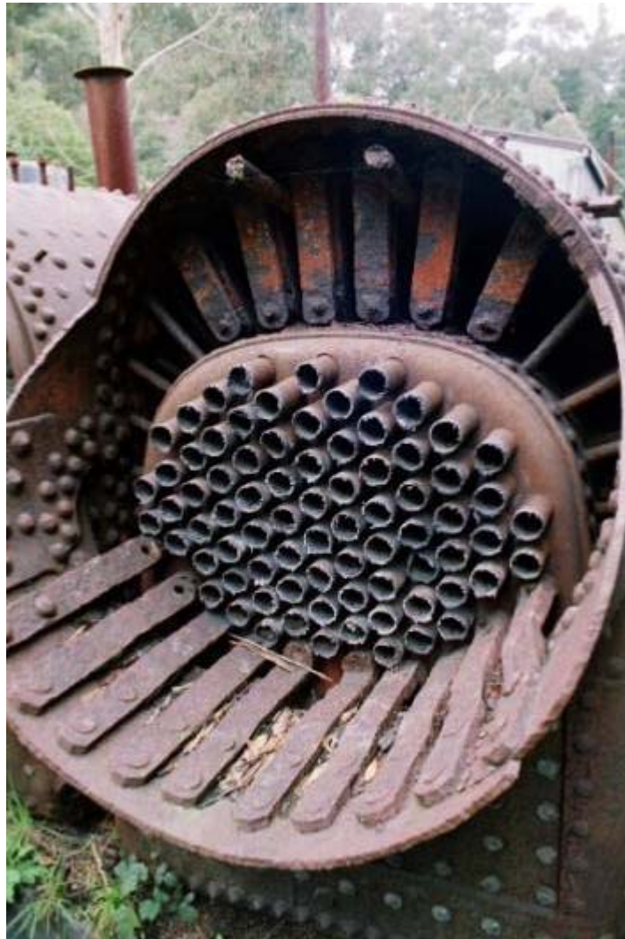
This is a photo looking from within the boiler, viewing back toward the rear flue sheet and firebox. You can see the arched shaped firebox slung within the boiler shell. Note the firebox stays holding the firebox in place, rigid stays to the sides, flexible pin jointed stays around the top.. Also note the boiler flues cut off as this old 1920s boiler once used on a 30" gauge Baldwin outside frame 2-6-2, awaits scrapping. Puffing Billy Railway, Australia.
