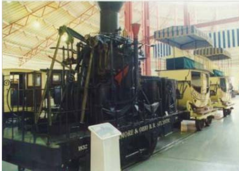
A typical early B&O Grasshopper loco - 1832. The main power of the B&O for the first 7 years B&O Museum Mt Clare. Baltimore.
