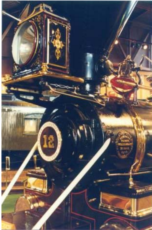
The typical Oil Box Headlight and mounting bracket of Baldwin's 1870s. The headlights were made by a specialist contractor to the Railroad.
