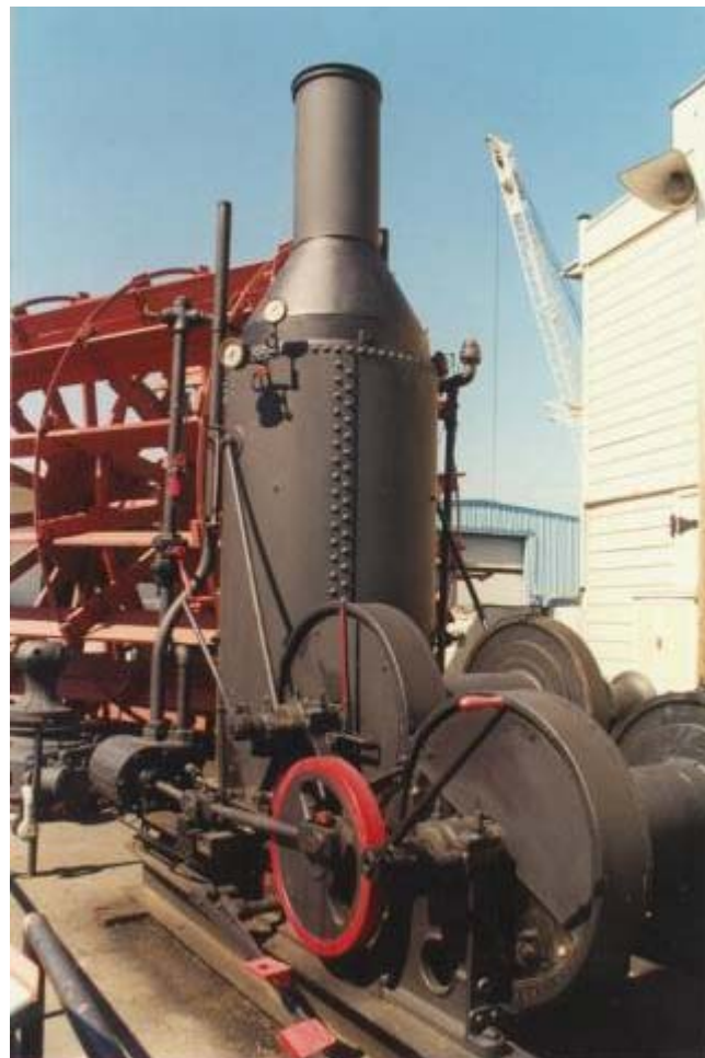
Typical Steam winch, as used in lumber, shipping, ski resorts and all kinds of applications, note the Cooper Vertical Boiler, Photo Taken at San Francisco Maritime Museum.
