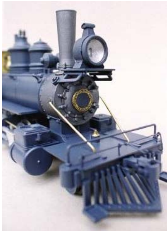
The 1.5mm Brass braces in place, ready for painting.
