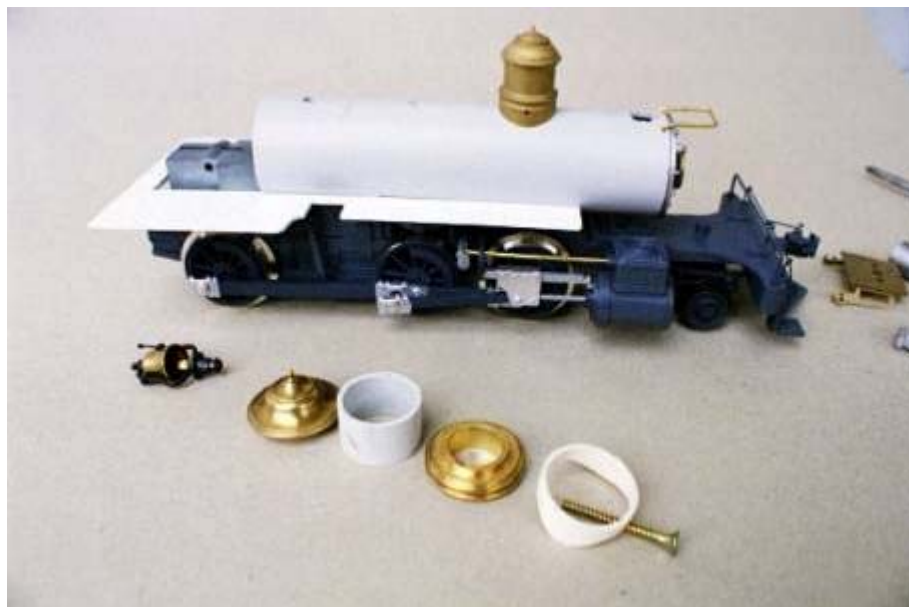
This picture shows all the steam dome parts lined up. The 33mm PVC dome base, the Aristo brass dome base, the 15mm tall 29mm dia. PVC cylinder and the brass dome top.
