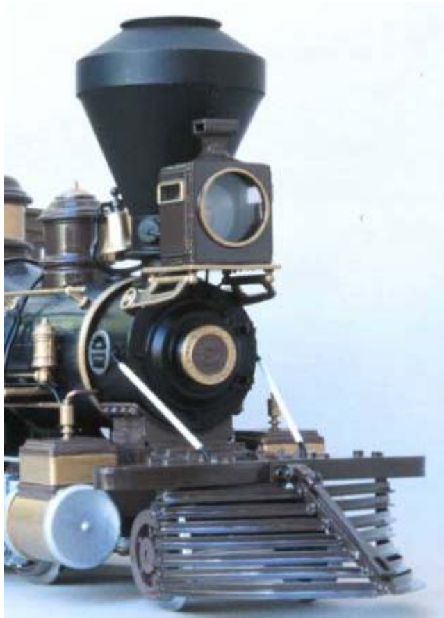
This is a typical Baldwin saddle with 4 bolt heads to both sides of the saddle.
