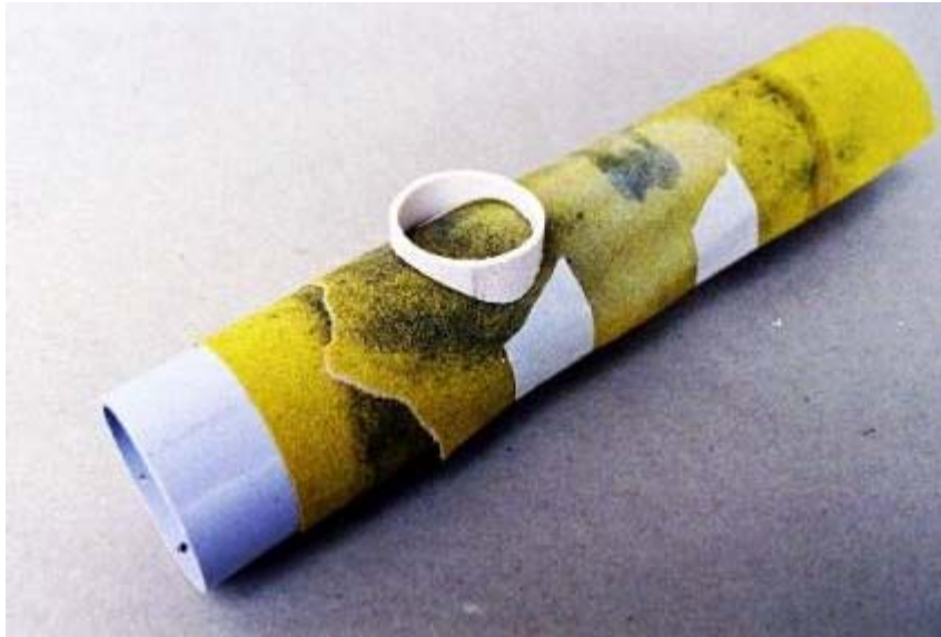
The 43mm PVC pipe clad in sand paper and my dome base being sanded to the right profile by grinding the thing back & forth over the pipe!!
