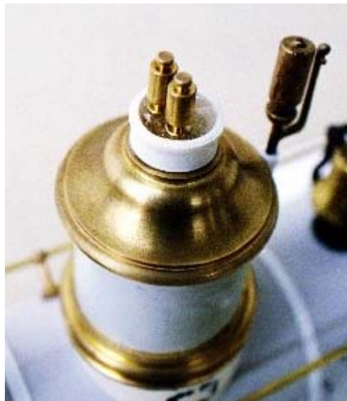
In this picture you can clearly see the two safety valves glued into a pool of araldite within the steam dome cluster. The whistle is mounted behind the dome.
