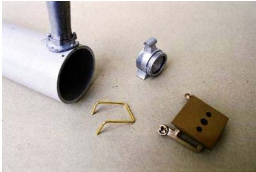
The above picture shows our false bracket made from 1.5mm brass rod, and the two holes in the front of the boiler where the bracket will be inserted.
