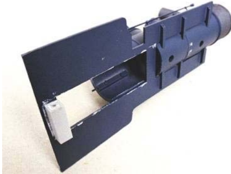
The 9x9 SHS block mounted to the rear underside of the cab floor
