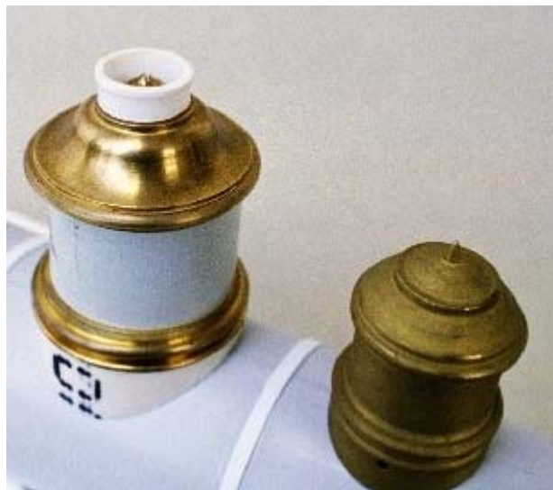
Here is the finished steam dome sitting on the boiler, sand dome in front.
