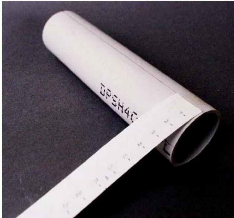
Note the upper datum line and the paper ruler taped to the datum used to mark out the lower datum under the boiler.
