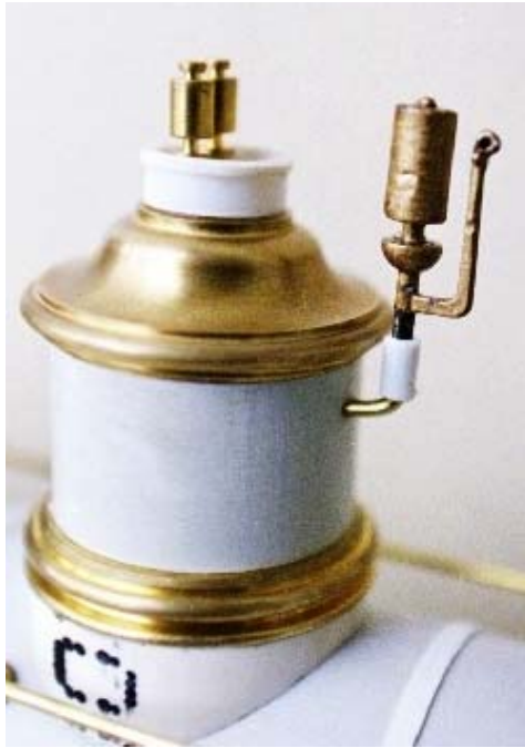
The whistle mounted to the rear face of the dome.
