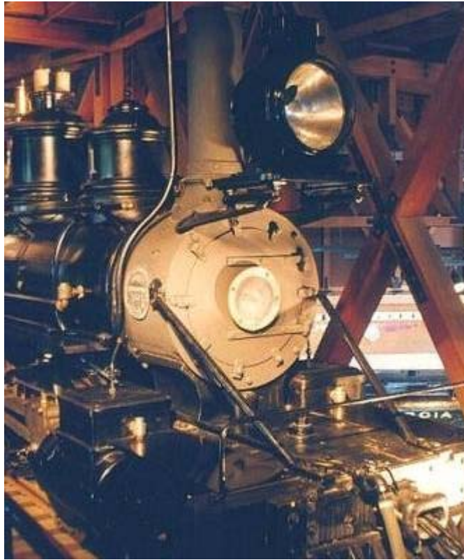
Note the disk like tops to the braces fixed to the smoke box sides and the flattened lower ends with two bolts at the pilot deck.
