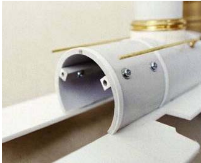
The boiler washout plugs (bolts) and Plastruct SHSs within the boiler.
