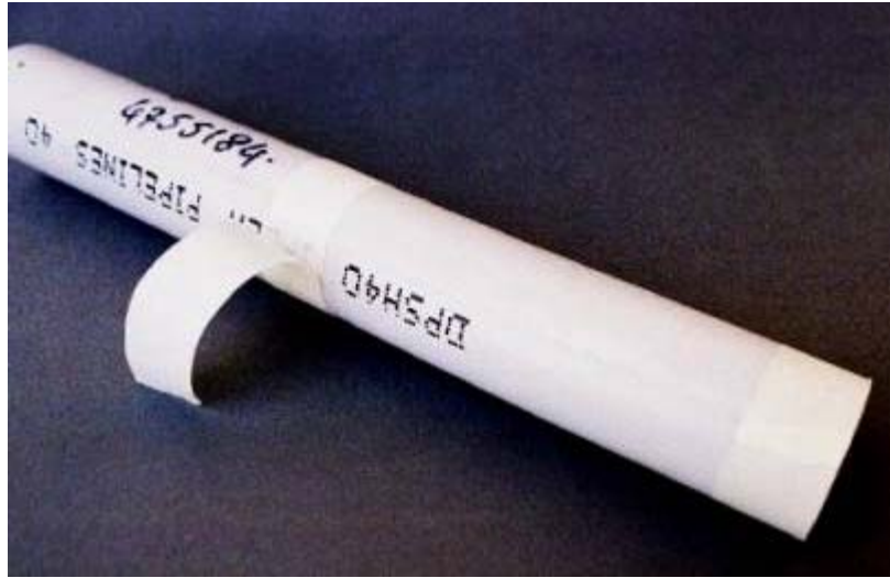
Cutting along evenly placed masking tape to guide a straight cut.
