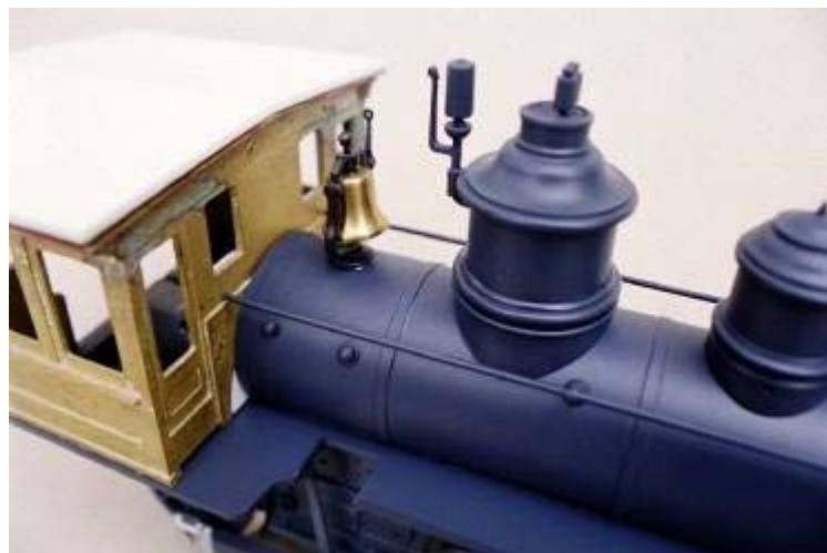
The boiler plugs seen fully painted as part of the boiler. Note the screwdriver recess in the bolt heads filled smooth with araldite.
