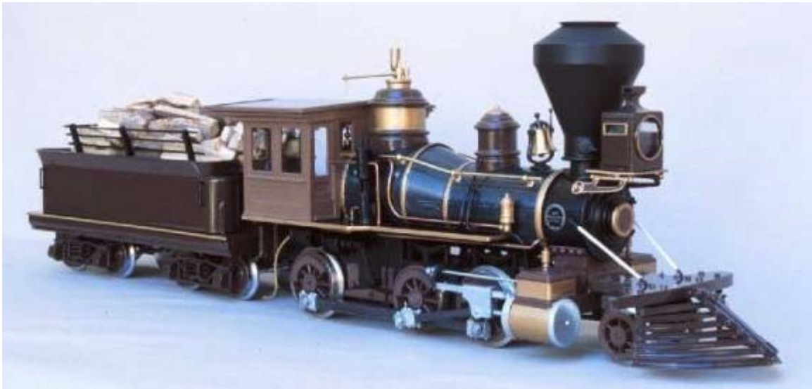
Painted 2mm styrene boiler bands.
