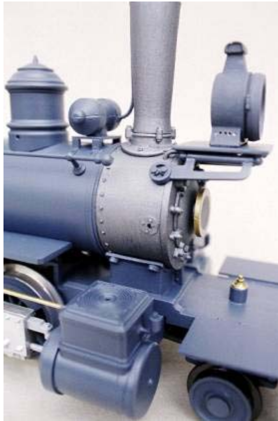
Rivets along rear end of smoke box.
