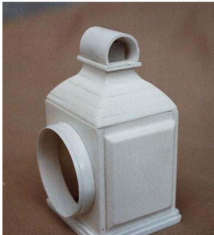
The layers of the crown evident in this unpainted headlight. Note the vent roof fixed into place.
