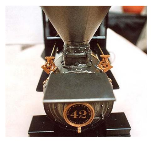
...a view from below the hand rail, see how it passes through the bell rig to the steam dome stub stanchion..
