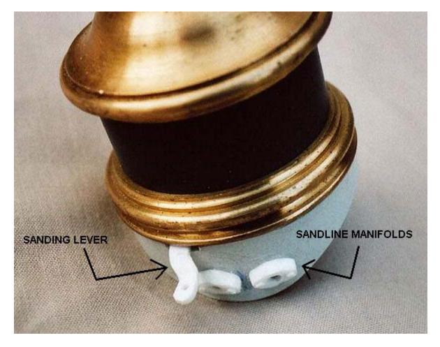
Note in the next picture the finished dome, featuring sand dome cap, 'final', sanding lever and manifolds and holes drilled through the dome base only in my forward manifolds (1885 Mason!).
