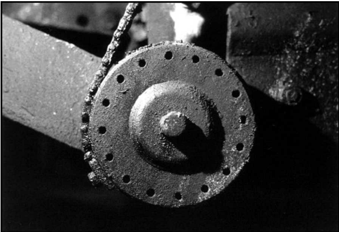
A close up of the real Johnson Bar spring as seen on the Torch Lake, note the use of the thin chain bolted to the 8 O'clock position on the disk.
