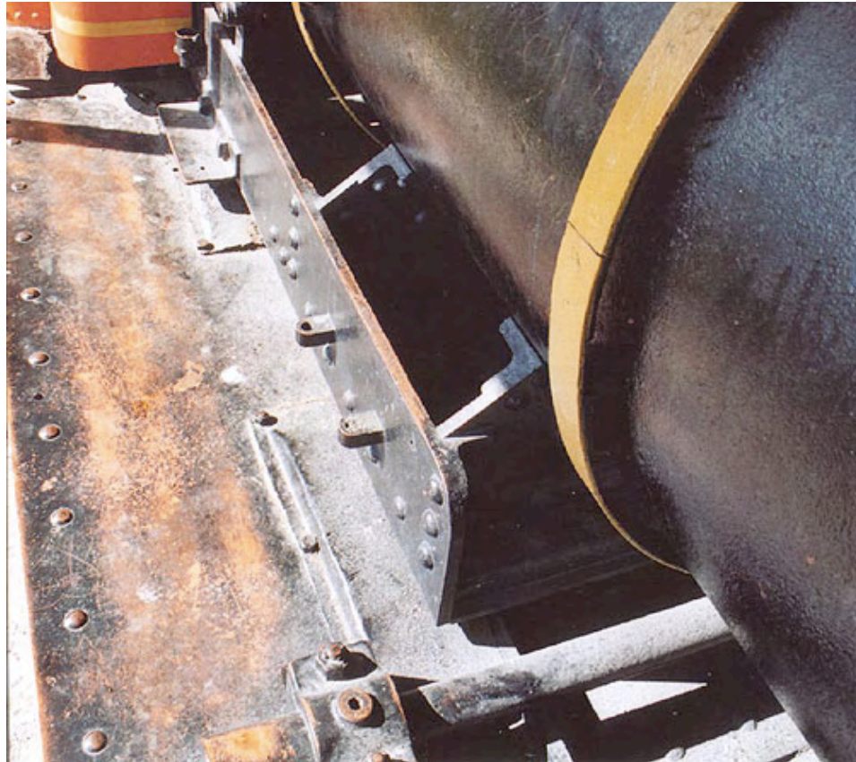
A close up of the boiler framing to which the pivot is mounted. Compare this is the rusty bearing plate of Torch Lake, as seen in Rich's photo above.
