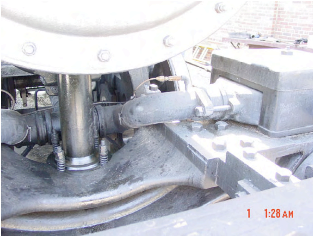
A view under the smokebox. The steam supply pipe can be seen coming from the middle chassis area, then splitting into a "Y" branch to the cylinders. The shiny vertical pipe is the steam exhaust pipe, which enters the smokebox via a crafted slip joint.
