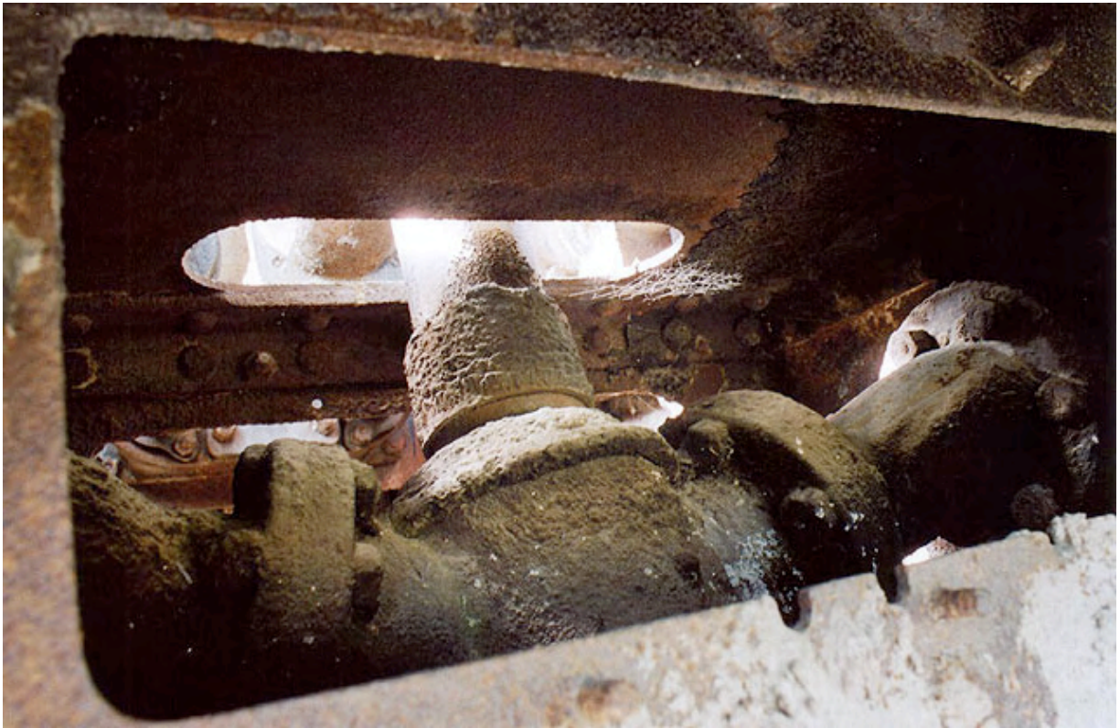
A view directly between the cylinders showing the steam exhaust lines from the two cylinders, converging into the vertical pipe to the smokebox above. Note how the vertical pipe exits the chassis deck via an elongated hole. Where Torch Lake uses a slot in the smokebox, this Fairlie's exhaust pipe also pivots via ball and socket joints.
