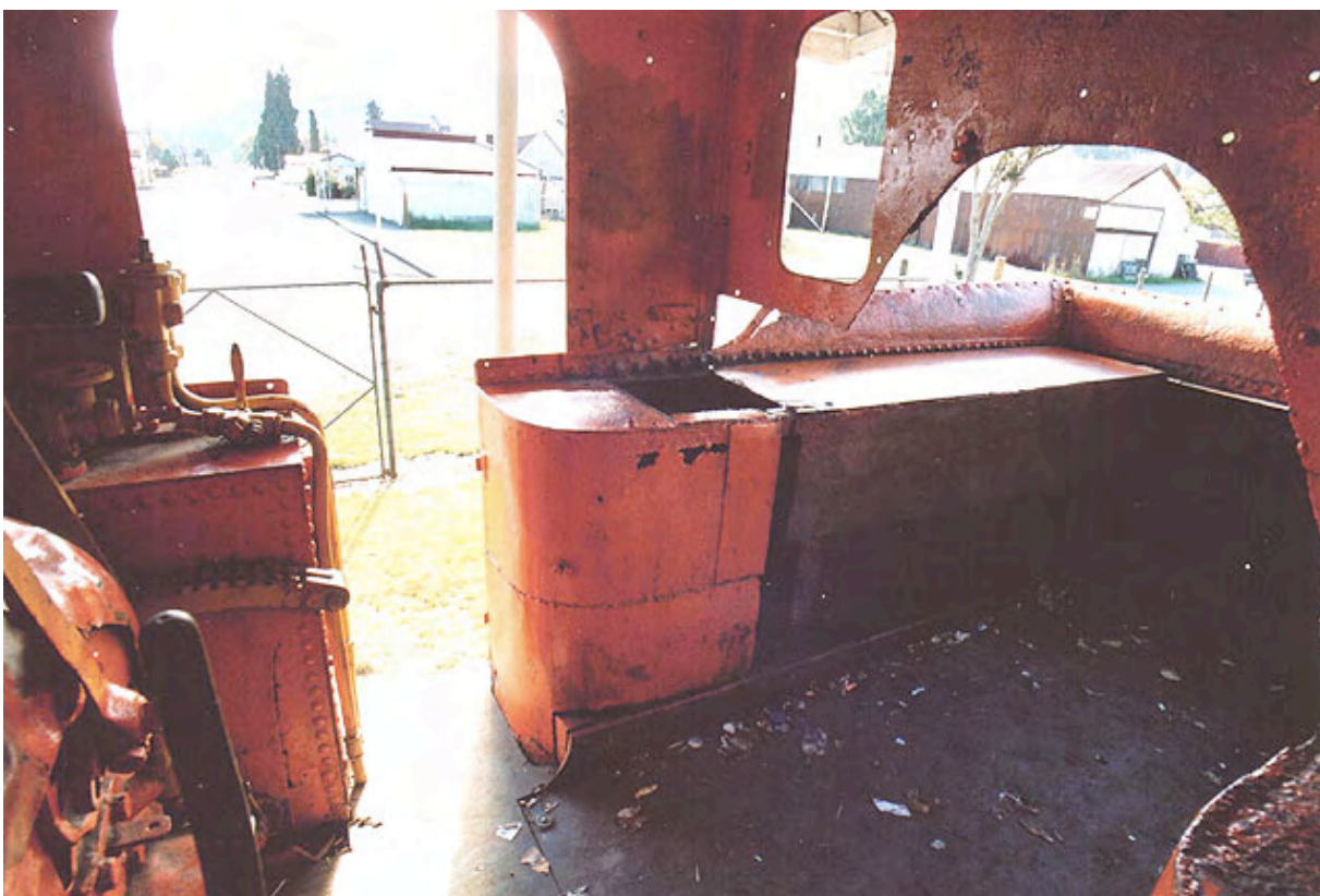
Note how the tender enters the cab in the same way as done by William Mason.
