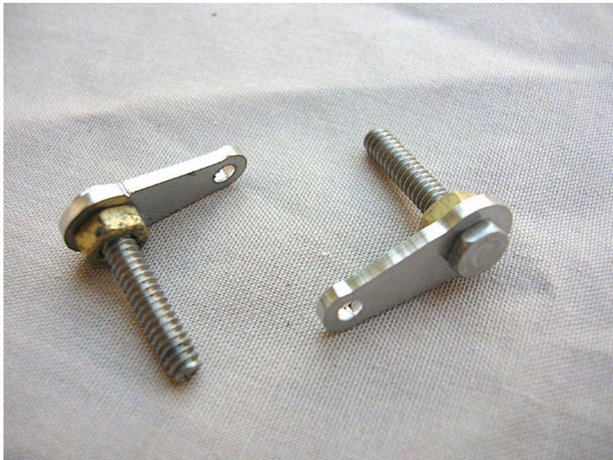
Two eccentric cranks ready for installation onto the 3rd Driver wheels.
